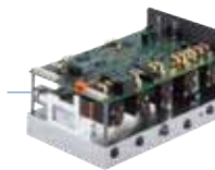
Five channel gas controller, featuring one common electronic board only
