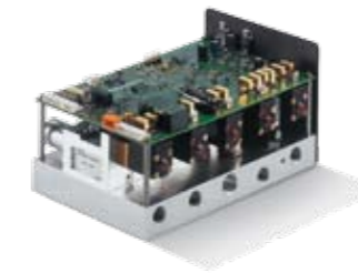
Electronic five channel gas blender
